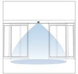
Wall mounting above sliding or revolving door
